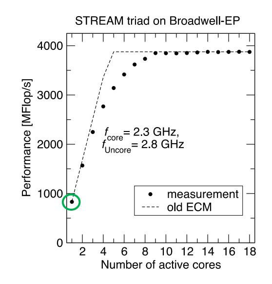
ECM is a resource-based model for the runtime of loops on one core of a cachebased multicore CPU
