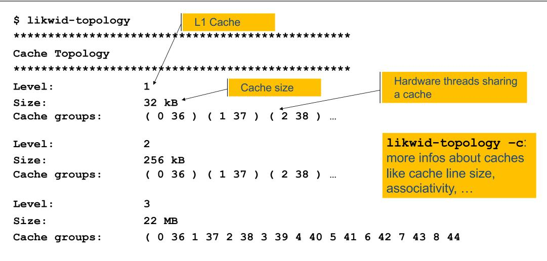
How many HW threads does your compute node provide?
