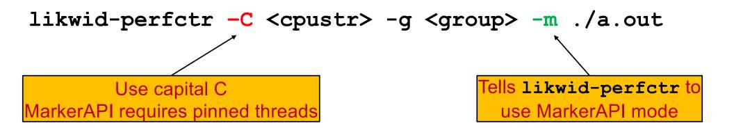
Copy perfctr/pi.c to marker/pi.c Add MarkerAPI calls around loop for each OpenMP thread & compile Measure the FLOP rate from 4 to number of phys. cores per socket
