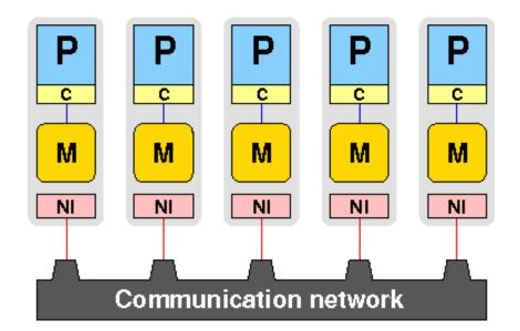
Data exchange and communication between processes is done by explicitly passing messages through a communication network
