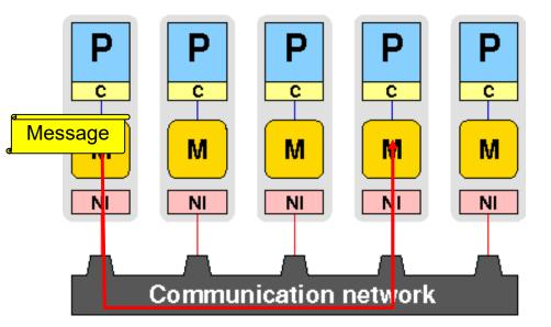
Data exchange and communication between processes is done by explicitly passing messages through a communication network
