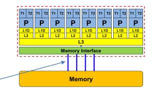
Typical memory bandwidth (20 cores): 160 Gbytes/s = 1.6 · 10<sup>11</sup> Bytes/s
