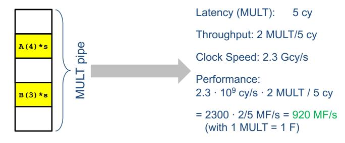
Single core on Intel Xeon E5-2695 v3 ("Haswell") with clock speed fixed to 2.3 GHz
