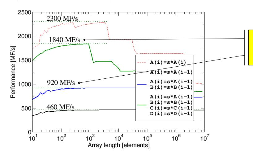
Increasing number of "independent dependencies" (i.e. increasing parallel workload) improves pipeline throughput
