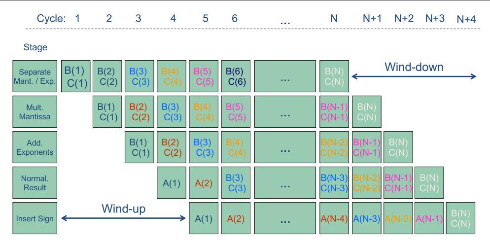
First result is available after 5 cycles (=latency of pipeline)!
