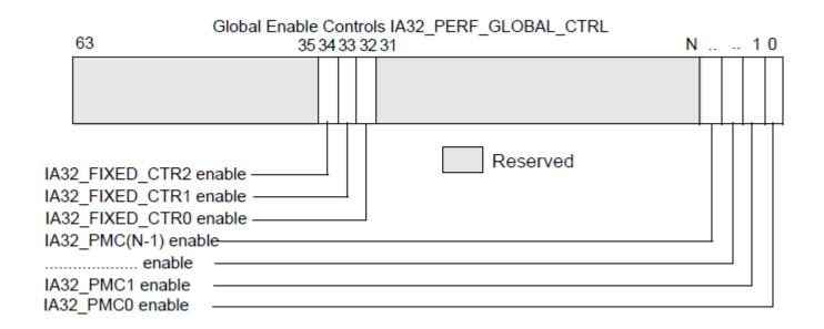
Global overflow registers (signal & reset) use same bit offsets
