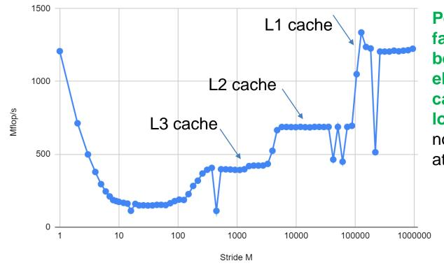
Performance drops by a factor of about 1/M initially because only every Mth element is used but all the cache lines still have to be loaded Beyond M=8 there is no strong change any more at first.
