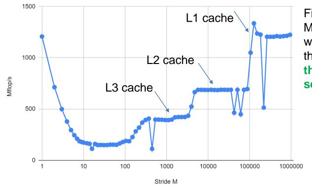
Finally, the last sharp rise at M=100000 indicates a working set of 64 kB, while the L1 size is 48 KiB, hence this is where the working set fits into the L1 cache
