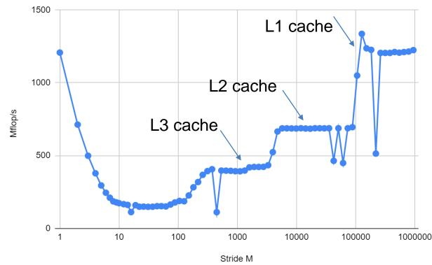
Behavior for larger M (blue dots): Starting at M=300 there is a **rise** in performance. At M=300, only every 19th CL is loaded (adjacent CL prefetch!). This is a working set of 108 (elements) x 8 bytes /  $19 \approx 42$  MB. The L3 cache of the Ice Lake CPU is 54 MiB, so the complete working set fits into the L3 at this point.
