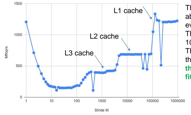
The second sharp rise is at about M=4000. Here, only every 500th CL is loaded. The working set is 8 x  $10^8$  bytes /  $500 \approx 1.6$  MB. The L2 size is 1.25 MiB, so this is near the point where the complete working set fits into the L2 cache
