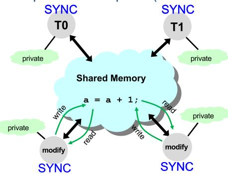
Synchronization: All threads need to wait until last thread enters synchronization
